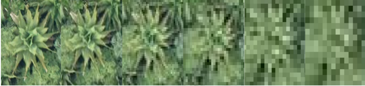
Figure 5.3: Resolution in cm/pixel from left to right: 5, 20, 40, 60, 80, 100. It is clear that after 60 cm/pixel the image becomes indiscernible.
