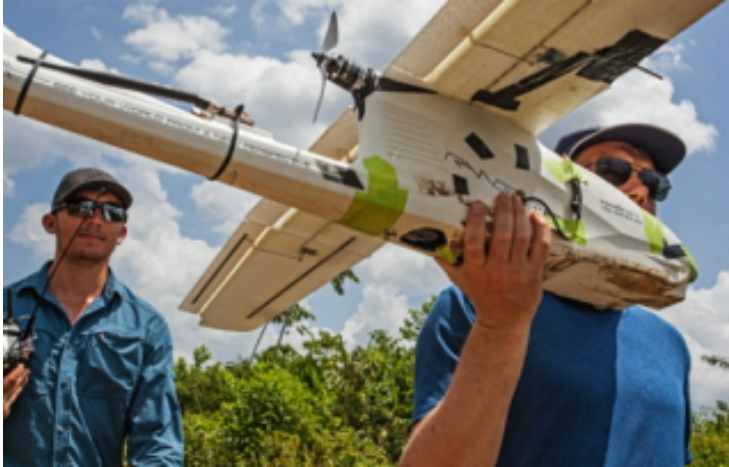
Figure 3.3: Volantex Ranger Ex about to be hand launched for its last day of data collection. The platform is easily managed by a team of two people and can be launched without out external equipment making it an ideal platform for difficult to access areas.
