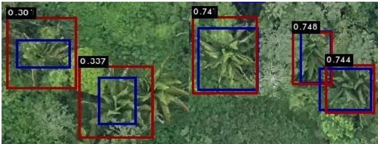
Figure 4.5: Example of IOU scores where blue corresponds to the human box and red corresponds to network detections.
