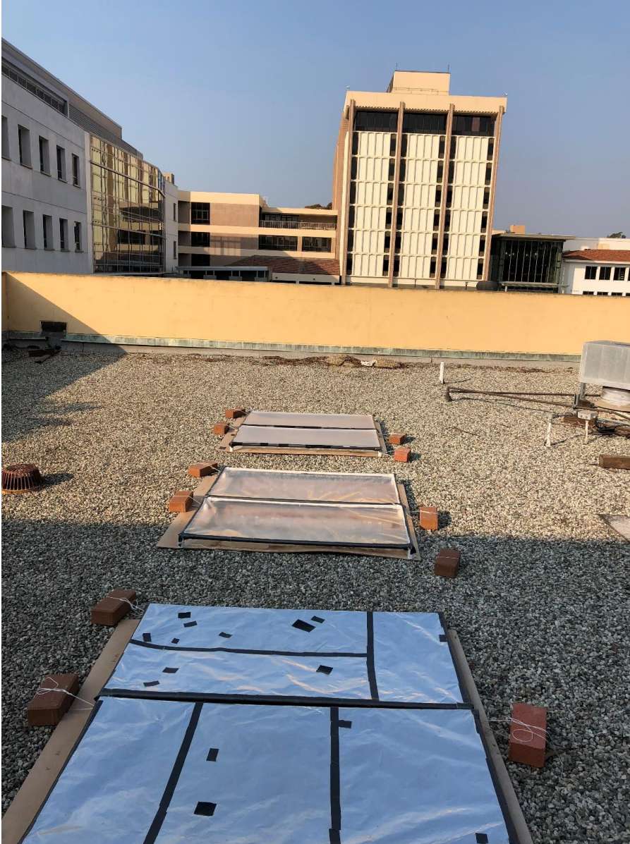
Figure A1-3: The outdoor experiment, during morning. All three radiation treatments are visible; each consists of two screens adjacent to each other, and sample bags are affixed to the wooden boards beneath the screens. See figure A1-1 for a close-up view of a sample bag affixed to one of these boards. The treatments, in order from closest to farthest, are the Radiation Block treatment, the UV + Visible treatment, and the Visible Pass treatment. Bricks were used to weigh down the screens and keep them in place. In the morning, the
