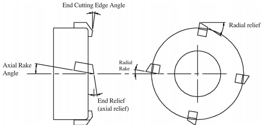
Fig. 4 Face milling cutter geometry
