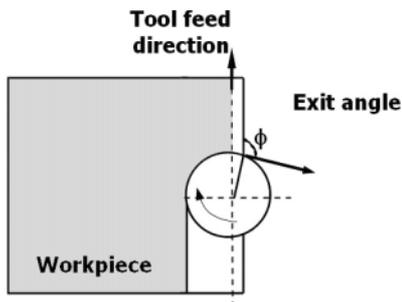
Fig. 3 Tool in-plane exit angle
