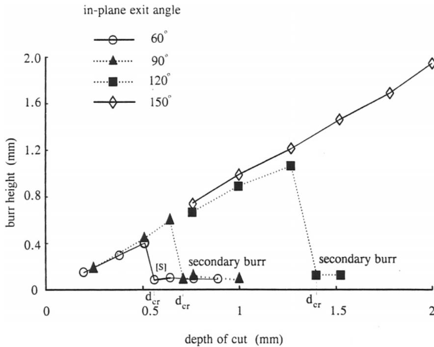
Fig. 2 Variation of burr height versus depth of cut and the exit angle for Al 6061-t6 [9]
