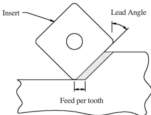
Fig. 5 Face milling cutter geometry: lead angle
