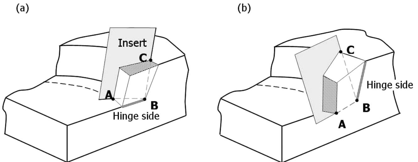
Fig. 6 Tool exit order sequence affects the burr formation condition [12]
