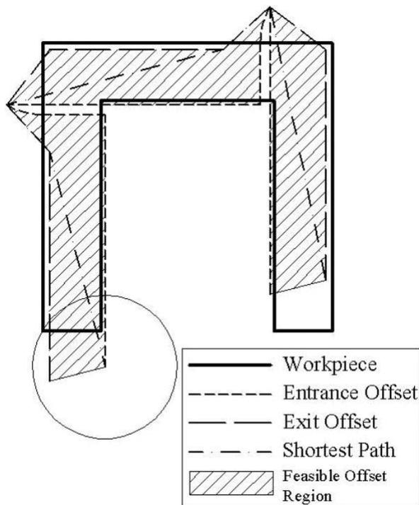
Fig. 10 Burr minimization using the feasible region approach on a sample part [20]
