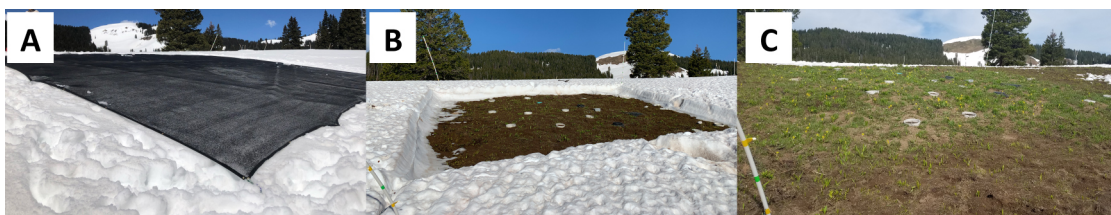
Figure 1. Visual representation of tarp deployment and resulting accelerated snowmelt during spring 2019 manipulation. A. The geotextile fabric was deployed after an isothermal snowpack was established. B. Removal of the tarp reveals the clear influence of this protocol on enhanced melting in the target plot. C. Contrast of the accelerated snowmelt plot with the control snowmelt reveals localized, accelerated onset of plant growth in the manipulated plot. Note, white rings visible within the area of manipulation were used for a separate experiment and are not discussed in this protocol (B, C).
