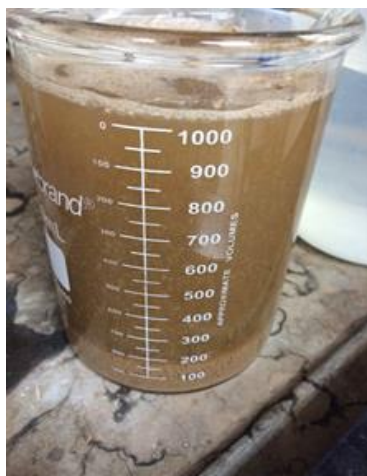
Figure 4.4 Lignin precipitated on the flask bottom by dilution of 1 part of hydrolyzate with 4 parts of water by weight.
