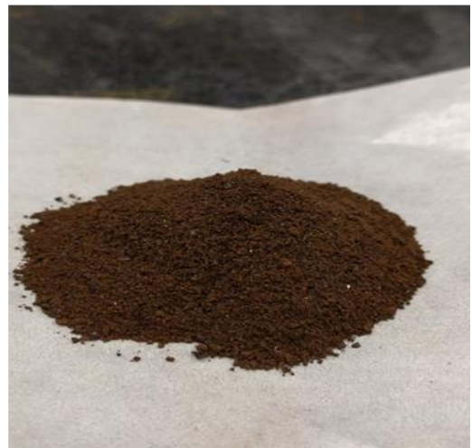
Figure 4.6 Lignin precipitated by dilution (left) and boiling (right), for fuel precursors case.
