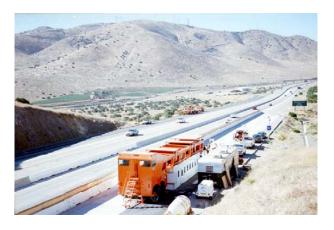
The Heavy Vehicle Simulator (HVS) testing program was initiated with a pilot study at the UCPRC Richmond Field Station. This included the evaluation of various types of instruments, methods of data recording, and the logistics involved with placing concrete around sensitive instrumentation. After the slab was cast, the HVS was used to evaluate performance of the various instruments as well as the performance of the slab under
