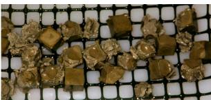
In the aggregate reaction study, alkali-silica reactions (ASR) were investigated in an accelerated test (ASTM C1260) in which mortar bar length changes were used to indicate potential reactivity. Two aggregates, granite (mildly reactive) and phyllonite (highly reactive), and five proprietary cements from four different manufacturers were used in the tests. Cements included:
