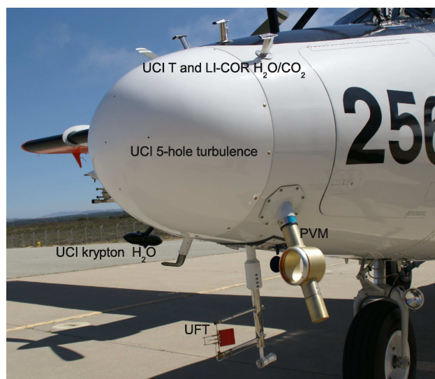
Fig. 1. Radome of CIRPAS Twin Otter research aircraft with fast-response instruments used in POST.
