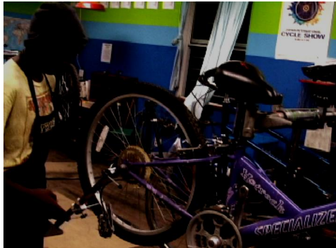
Figure 5-6. Marcus explores the geometry of parallel planes in advance of discovering the relationship between a misaligned derailleur hanger and derailleur dysfunction.
