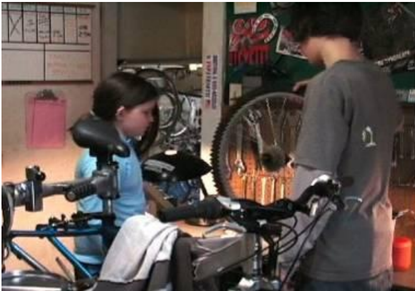
Figure 6-1. Emily and Josh in the Cascade shop discuss a strategy for overhauling a rear wheel, which Josh is holding in his right hand. The first step involves removing the freewheel, a cluster of cogs visible at the center of the wheel.
