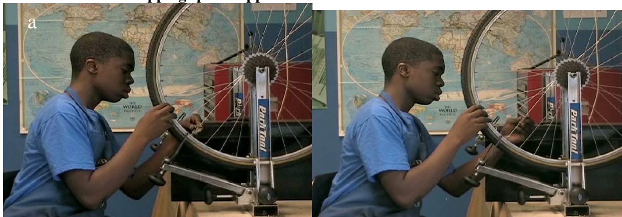
Figure 6-1. Marcus truing a wheel at the truing stand: (a,b) a sequence showing the subtle movement of Marcus's left hand downward along a spoke indicating his careful technique intended to avoid stripping spoke nipples.
