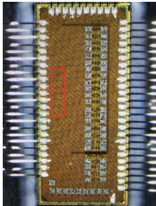
Figure 9. Die Photo of TDC evaluation prototype. Clock receivers are in outlined area.
