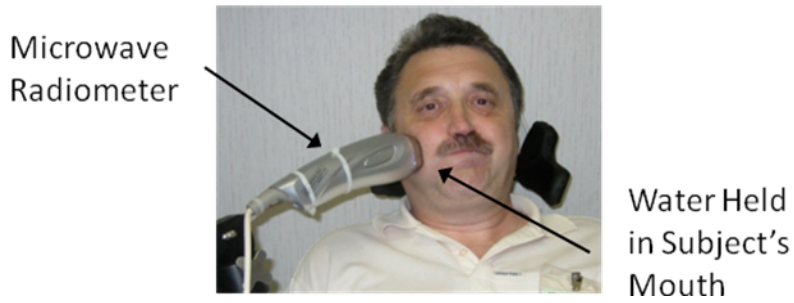
Figure B.5. Experimental setup for the measurement of water temperature in the mouth
