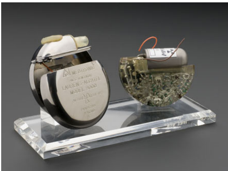
Figure 1.11. Image of an implantable pacemaker with a radioisotope TEG as the power source [85]. The size of the pacemaker is about as large as a pack of cigarettes, which is much larger than today's pacemakers [91].
