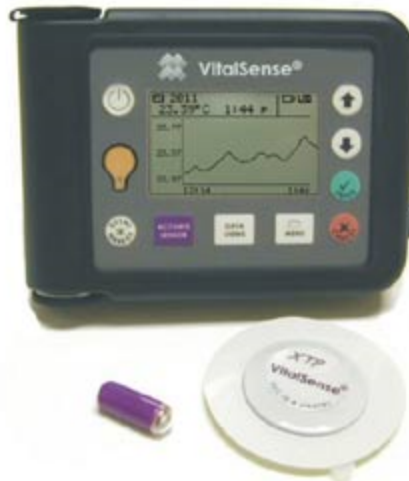
Figure A.1. Mini Mitter/Philips Respironics VitalSense Receiver with a temperature patch and capsule.
