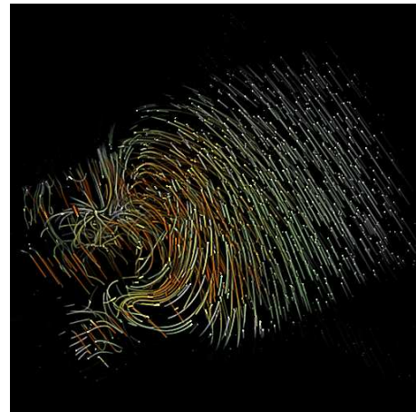
Figure 4: Animation with dense geometric flow visualization applied to unsteady flow of jets data set. Pathlines are rendered at time steps 1120, 1400, and 1800.
