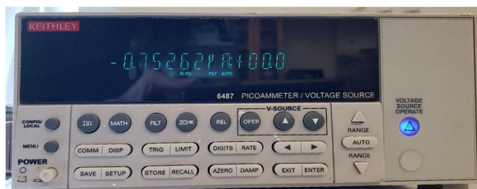
Figure 1.3: Image of Keithley 6487 picoammeter/voltage source used in etching as well as electrochemical characterization experiments.
