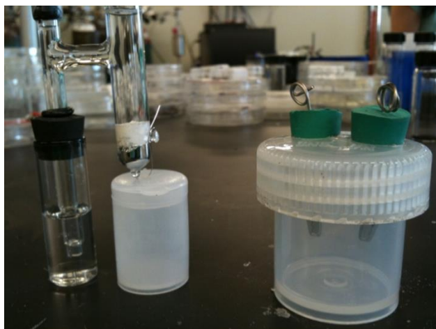
Figure 5.3.4: Experimental setup for linear polarization experiments. Saturated calomel reference electrode is on the left, testing cell is on the right.
