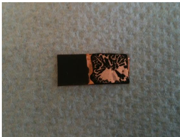
Figure 3.3.20: Effect of Ketjen black on physical properties of dried slurry. Deposited slurry on left has zero Ketjen black and slurry on right has 13% Ketjen black.
