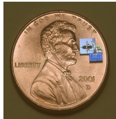
Figure 1.2.2: Smart dust mote can sense and communicate over a surface area of a few square millimeters. The device requires greater than 100 \text{ J/cm}^2 of energy to operate. [5]
