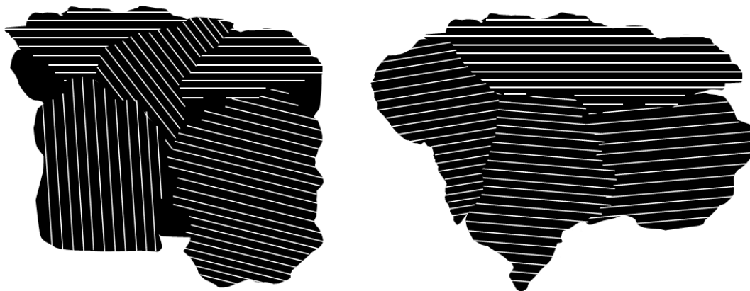
Figure 3.1.3: Structural difference between hard and soft carbon. Hard carbon exhibits high turbostratic nature and amorphous regions (left). Crystallites of soft carbon are closely aligned. (right)
