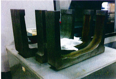
Figure 7: A photo showing the tuner arms that have been wire EDMed at the Fermilab machine shop.
