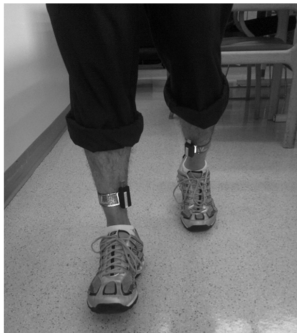
Figure. Accelerometers held firmly above the ankles.
