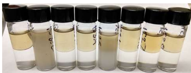
Figure 23: Phase separation upon extraction
