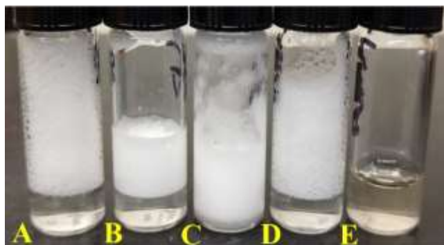
Figure 5: Shaken samples of 2 wt % surfactant aqueous solutions: (A) SDS, (B) PTS, (C) Nok, (D) TPGS-750-M, (E) Coolade
