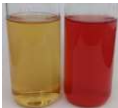
Figure 24: Left: Coolade 2 wt % solution stored under argon, Right: Coolade 2 wt % solution stored under air, showing decomposition
