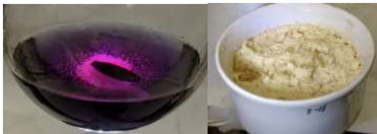
Figure 27: Reaction at completion, crystals filtered after precipitating with HCl
