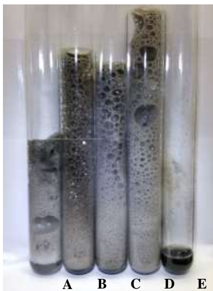
Figure 6: Foaming test using Fe/ppm Pd/Ni NPs using (A) SDS, (B) PTS-600, (C) TPGS-750-M, (D) SPGS-550-E (E) Coolade.
