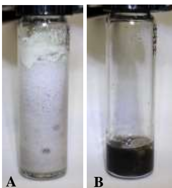
Figure 10: Reaction appearance (A) TPGS-750-M, (B) Coolade
