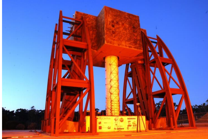
Figure 5.1: Full-scale reinforced-concrete bridge column tested on the LHPOST@UCSD
