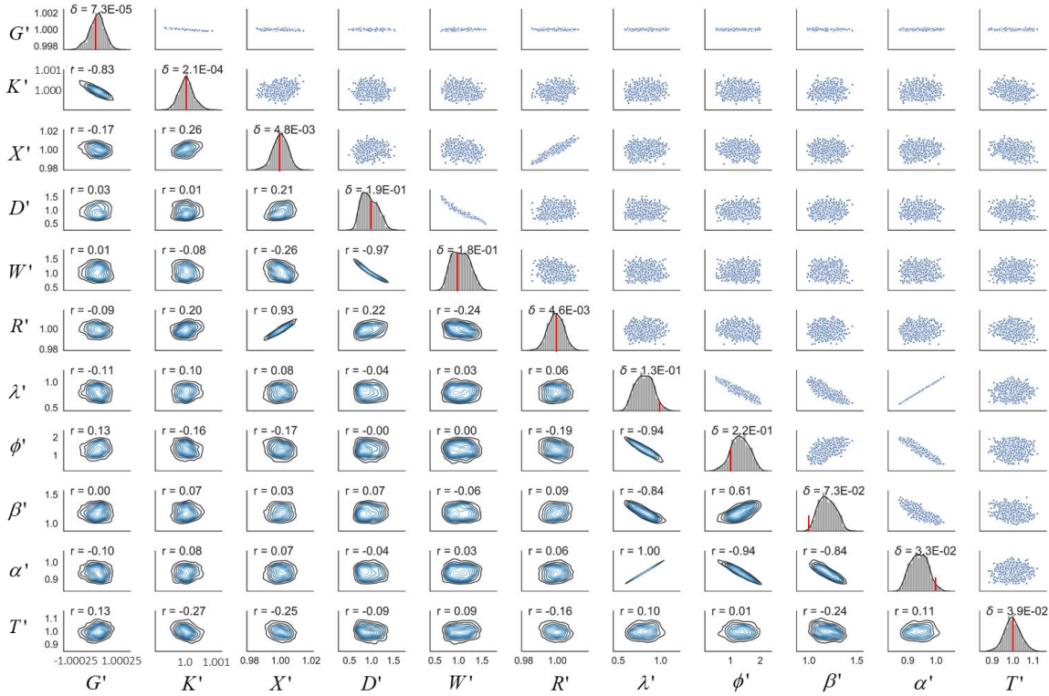
Figure 2.8: Pairs plot of eleven parameters of testbed structure obtained using posterior samples generated by TMCMC.
