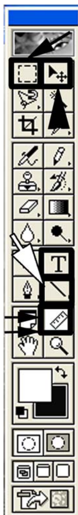
Fig. 1 The toolbar from the software package is shown with common tools needed for digital templating: line tool (white arrow); measure tool (small black arrows); text tool (letter T); marquee tool (black arrow); and move tool (large black arrowhead).
