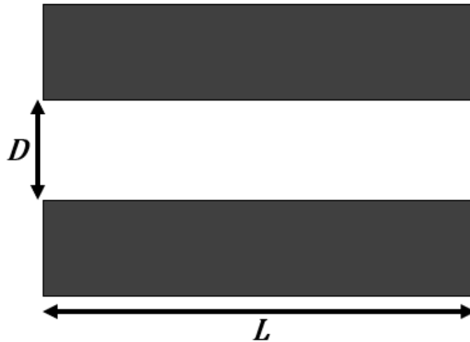
Figure 2.2: Schematic of the geometric definitions of a cylindrical pore, see eq. 18.
