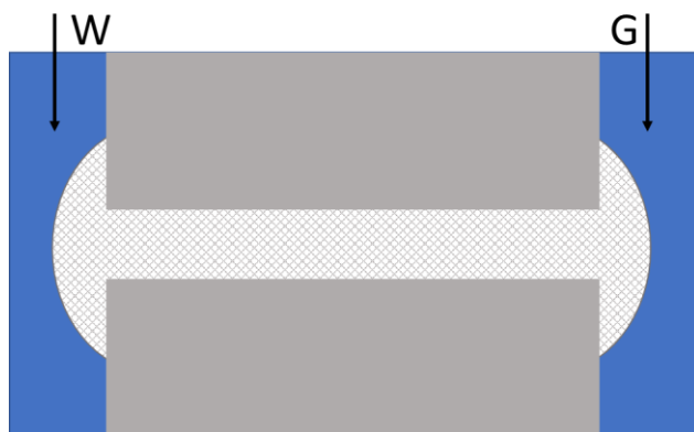
Figure 2.7: Single pore filled with ionogel placed in contact with an ionic liquid with lithium salt; two electrodes are placed in the liquid. The PET membrane is shown in grey, ionic liquid in blue, and the patterned region represents the casted ionogel. The arrows show the two electrodes labeled “W” for working and “G” for ground.
