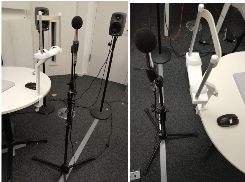
Figure 11: The speaker loudness calibration setup.
