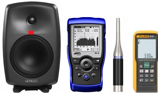
Figure 10: Genelec 8040 Studio Monitor with the reference point marked in Red according to [3], adapted from [4], SPL Meter NTi Audio, Model:XL2 and M4261 microphone [5], Fluke 424D Laser Distance Meter [6].
