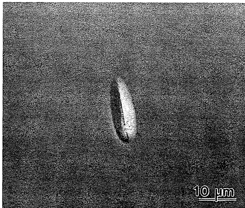
FIG. 1. SEM micrograph of an oval defect formed in MBE-grown GaAs (courtesy of Dr. Calawa, MIT Lincoln Lab.).
