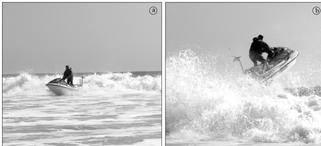
Figure 1.10: (a) Inbound and (b) outbound cross-shore transects through the surfzone with the jet ski mounted WS. (a) Inbound transect bubbles are minimized by driving just in front of a shoreward traveling bore. (b) On outbound transects, bubbly water is drawn into the flow-through WS system as the jet ski drives over a bore
