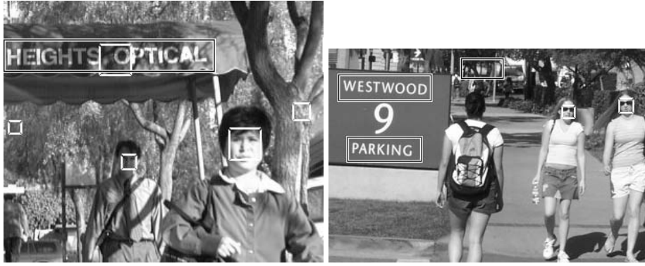
Fig. 11. The boxes show faces and text as detected by the AdaBoost log posterior ratio test with fixed threshold. Observe the false positives due to vegetation, tree structure, and random image patterns. It is impossible to select a threshold which has no false positives and false negatives for this image. As it is shown in our experiments later, the generative models will remove the false positives and also recover the missing text.
