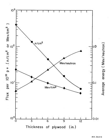
Fig. 1. Attenuation of Bevatron stray neutrons in plywood: two-counter study in experimental area.
