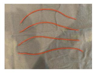
5. For each strand of electric wire, use a wire cutter to remove 1cm of insulation from each end.
