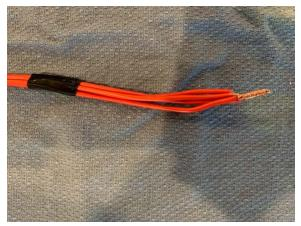
13. Attach one end of an alligator clip #1 to this bundle of exposed ends. Secure with electrical tape.
