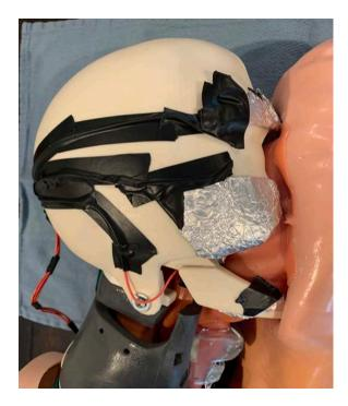
Secure the electric wire strands to the simulated skull using electrical tape. It is optimal to tape the right sided strands together into one "cord" and the left sided strands together into a separate "cord."
