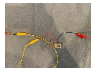
16. Attach the other end of alligator clip #2 to one electrode of the 9V battery.
