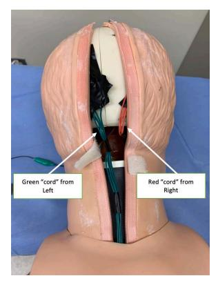
11. Carefully return the simulated skin to its original position, bringing it up and over the target zones. Alternatively, you may wish to leave this until the final step to ensure that all electrical connections are working properly.
