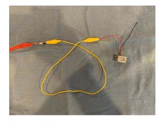
15. Attach one end of alligator clip #2 to the other end of the piezo electric buzzer.
