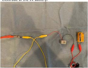
17. Attach one end of alligator clip #3 to the other electrode of the 9V battery.
