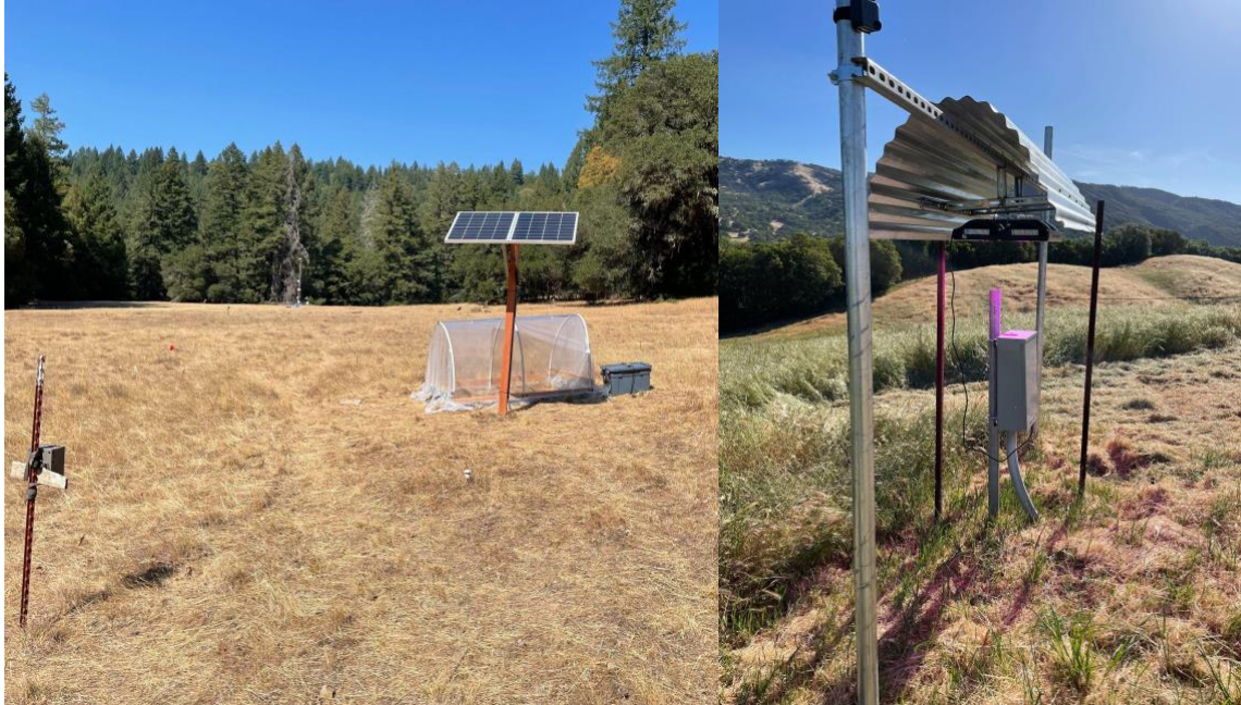
Figure 2. Central power source and treatment setups. Left: solar panel setup at ACRR with miniature greenhouse and small LED light bar. Right: Electrical box setup at HREC with high powered LED array.
