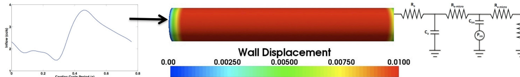
Figure 4.5: Typical coronary flow waveform applied at inlet and coronary boundary condition applied at outlet. Significant wall displacements are observed during systole.
