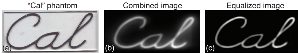
Figure 4.8: Experimental data on a “Cal” shaped phantom shows resolution and contrast improvement with equalization filter. (a) Photograph of a “Cal” shaped acrylic phantom. (b) Combined image from multichannel acquisition shows isotropic resolution and uniform channel width. (c) Equalization filter dehazes the image without amplifying noise, improving resolution and image quality.
