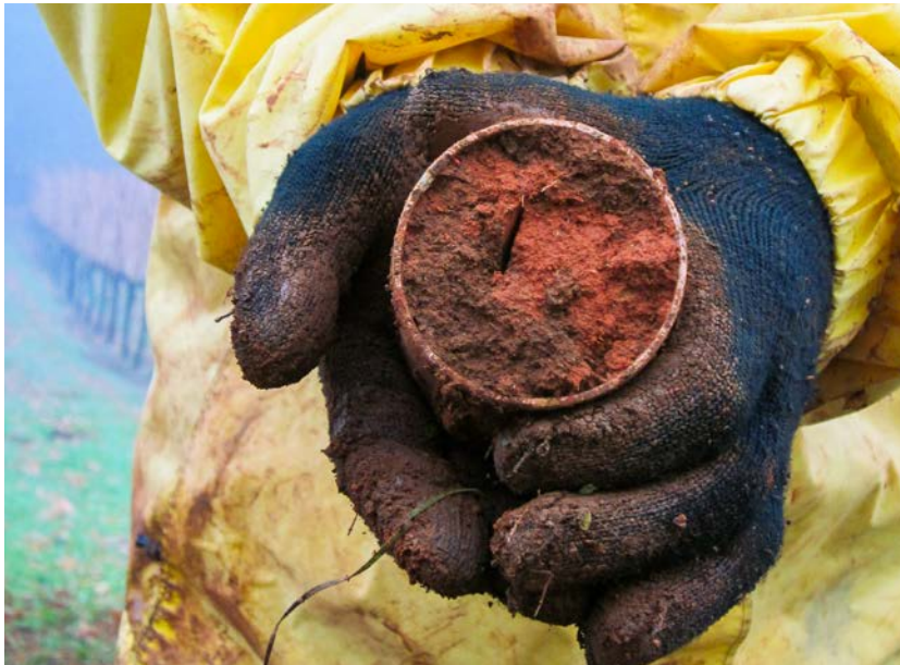
Soil core collected to measure bulk density in the subsoil of a vineyard alley in the Napa Valley. Photo: Kerri Steenwerth, USDA-ARS
