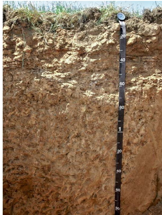
A soil profile from soil health region 3 showing a root-restrictive horizon between 30 cm and 50 cm relative to the black tape measure. Photo: Toby O'Geen
