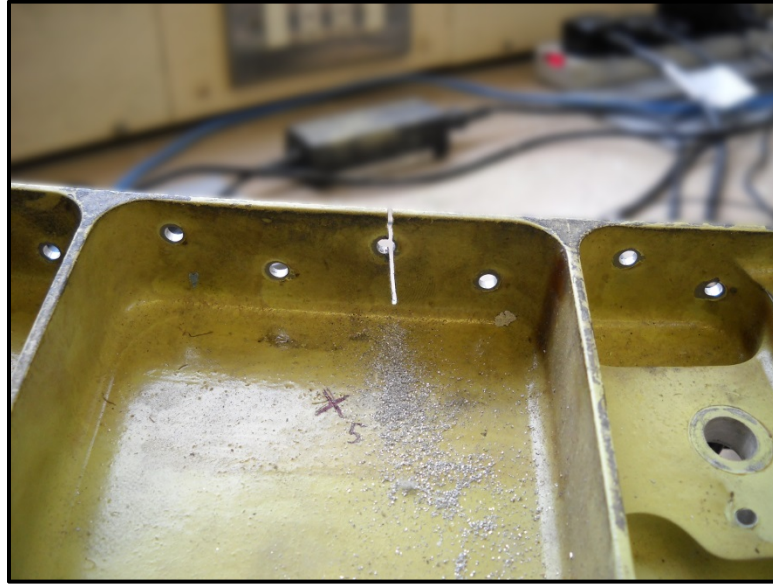
Figure 17 - Crack damage introduced in fuselage rib structure
