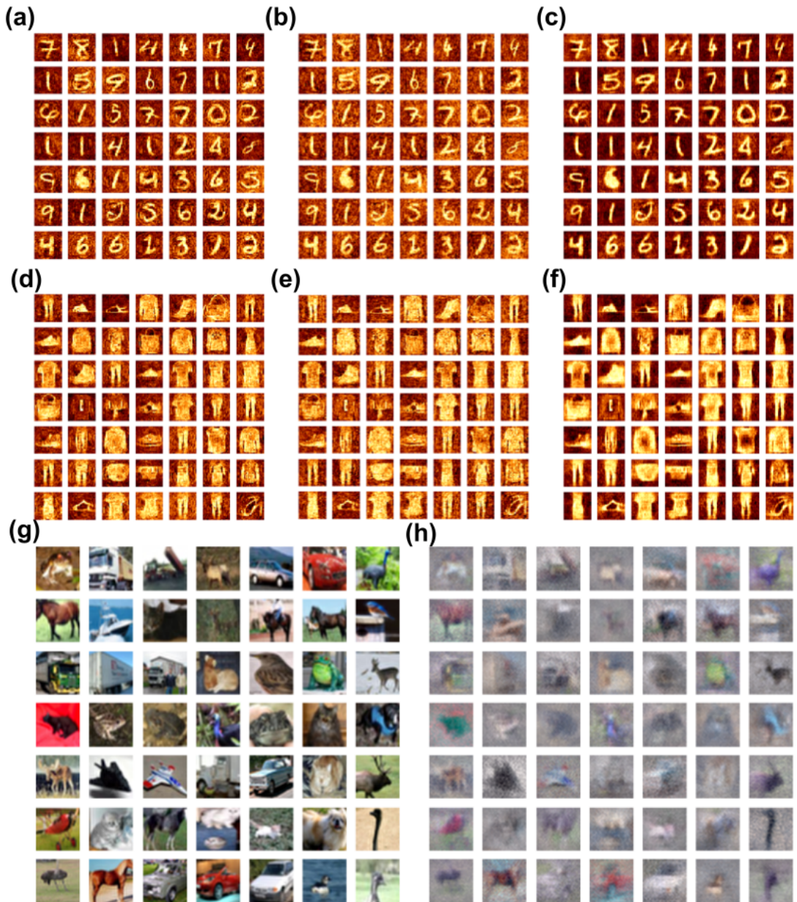
Figure 3.2: Reconstructed images from (a, b, c) MNIST handwritten and (d, e, f) fashion MNIST datasets with random, Fourier and vortex bases, respectively. The vortex basis provides edge enhancement for object detection. (g) Ground truth and (h) reconstructed images from the CIFAR-10 dataset using the vortex training bases and a vortex mask as the encoder.
