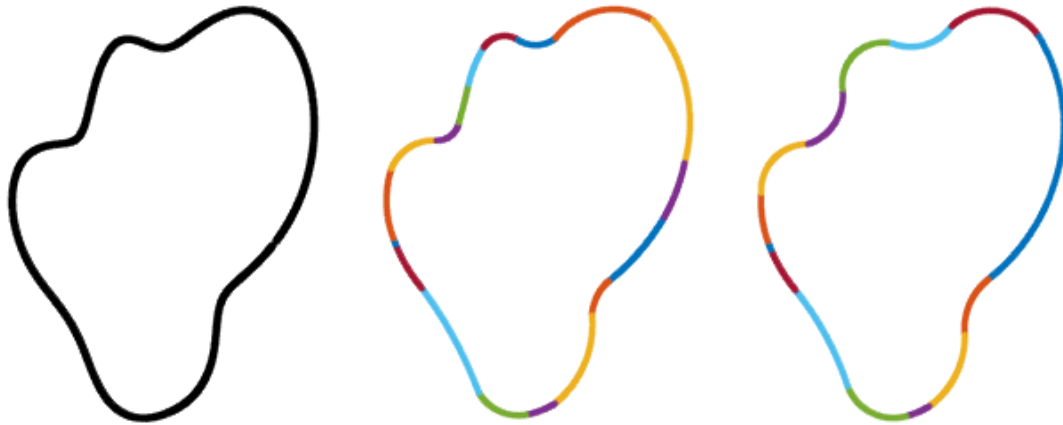
Figure 3. Two constant curvature representations of a shape contour. The original shape (left) is approximated with a small W (middle) and a large W (right). The smaller integration window has more segments and represents the contour more precisely.
