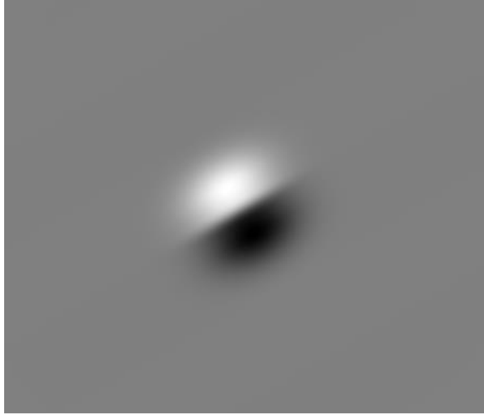
Figure 2. Sample odd-symmetric S-Gabor used in the detector model. The scale of the detector is increased for purposes of presentation.
