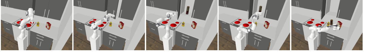
Figure 5.4. Snapshots of the trajectory planned using CVQ-MPT for the Panda Arm completing the multi-sequence task (from left to right). CVQ-MPT can plan trajectories for various types of planning constraints in complex environments.
