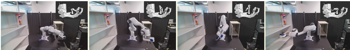
Figure 4.6. Snapshots of a trajectory planning using VQ-MPT for physical panda robot arm for a given start and goal pose on a shelf environment. On the top-right of each image, we show the point cloud data captured using Azure Kinect cameras. We used markerless camera-to-robot pose estimation to localize the captured point cloud in the robot’s reference frame. VQ-MPT can generalize to real-world sensor data without additional training or fine-tuning.
