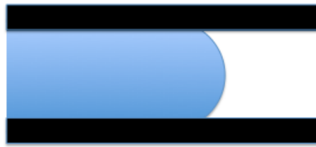
Figure 1.6: Schematic picture of capillary displacement method for forced spreading mechanism [20].
