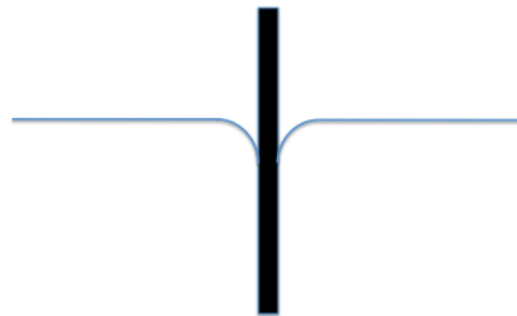
Figure 1.7: Schematic picture of Wilhelmy plate method for forced spreading mechanism [20].
