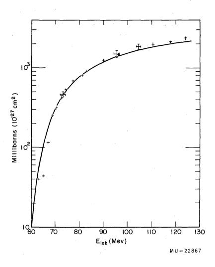
Fig. 9. Cross section for fission of  $U^{238}$  with  $C^{12}$  ions as a function of  $C^{12}$  energy. The curve shows the cross section for formation of the compound nucleus for a square-well model with a radius parameter of 1.5 x  $10^{-13}$  cm.
