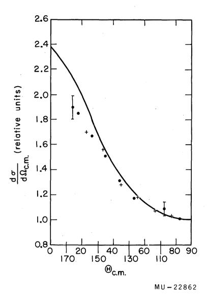
Fig. 4. Differential cross section of fission fragments from the reaction between  $U^{238}$  and 95.4-Mev  $C^{12}$  ions. The transformation to the system of the fissioning nucleus was performed with  $X_{\rm m}^2 = 0.018$ . The curve is theoretical (see text).
