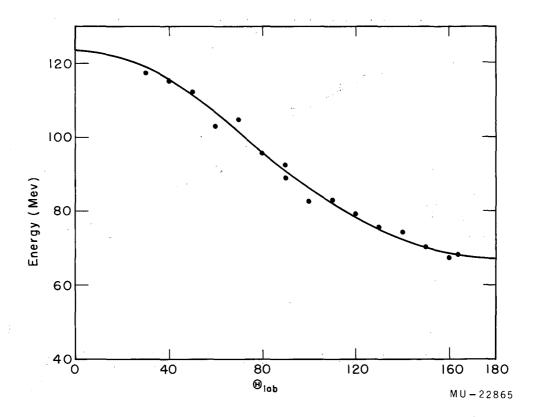
Fig. 7. Most probable kinetic energy of the fission fragments from the reaction between  $U^{230}$  and 95.4-Mev  $C^{12}$  as a function of lab angle. The curve is calculated for  $E_{\rm C}=93$  Mev and  $X^2_{\rm mp}=0.023$ . The points are experimental.
