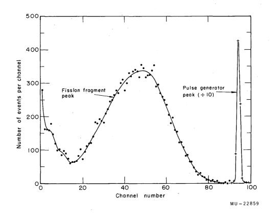
Fig. 1. Spectrum of fragment kinetic energies from fission of  $U^{238}$  induced by 124-Mev  $C^{12}$  ions. Observed at 90 deg to the beam with a p-n junction detector reverse-biased by 6 v.
