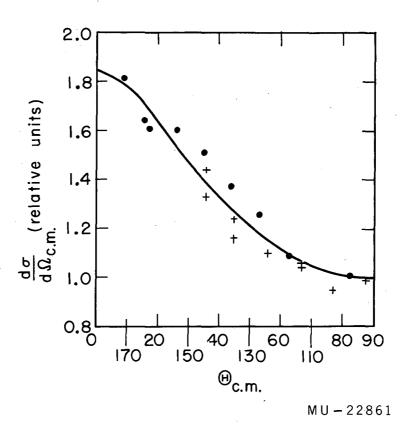
Fig. 3. Differential cross section (in the system of the fissioning nucleus) for fission fragments from the reaction between  $U^{250}$  and 73-Mev  $C^{12}$ ;  $X_{\rm m}^2$  = 0.018. The curve is calculated (see text).
