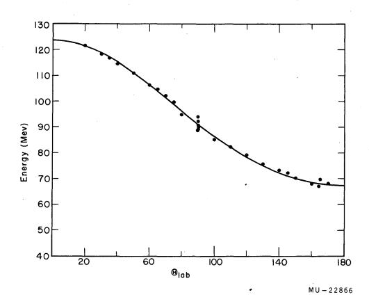
Fig. 8. Most probable kinetic energy of the fission fragments from the reaction between  $U^{230}$  and 124-Mev  $C^{12}$  as a function of lab angle. The curve is calculated for  $E_{C}$  = 93 Mev and  $X_{mp}^{2}$  = 0.023. The points are experimental.
