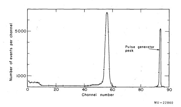
Fig. 2. A typical spectrum for 73-Mev C  $^{12}$  ions scattered from UF  $_{l_{\downarrow}}$  at a scattering angle of 25 deg in the laboratory system. Observed with a p-n junction detector reversebiased by 9 v.
