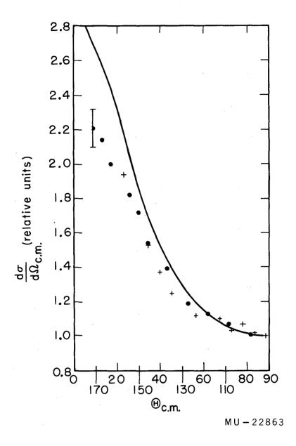
Fig. 5. Differential crass section of fission fragments from the reaction between  $U^{230}$  and 124-Mev  $C^{12}$  ions. The transformation to the system of the fissioning nucleus was performed with  $X_{\rm m}^2 = 0.022$ . The curve is theoretical (see text).
