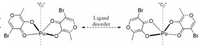
Figure 4. Schematic of the ligand disorder in the Pu(L 2 ) 4 crystal structure. The generated “pseudo-C 2 ” axis is indicated and the shorter Pu-O(phenoxide) bonds in each configuration are indicated in bold. Only one ligand pair is shown here, but the same disorder is seen in the other pair of ligands.
