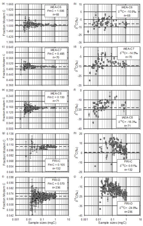
Figure 3 Secondary standards: fraction modern carbon and  $\delta^{13}C$  results for all IAEA standards, FIRI-C, and -D samples between  $\sim\!0.002$  and  $\sim\!1$  mg C from multiple  $^{14}C$  AMS measurements. All results have been corrected for MC and DC contamination (blank subtraction formulas given in Santos et al. 2007a) as well as for isotopic fractionation with on-line  $\delta^{13}C$  AMS values.
