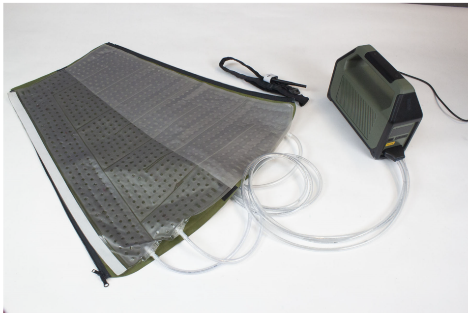
Figure 3. Photo of limb-cooling device chiller and sleeve with dot welds.
