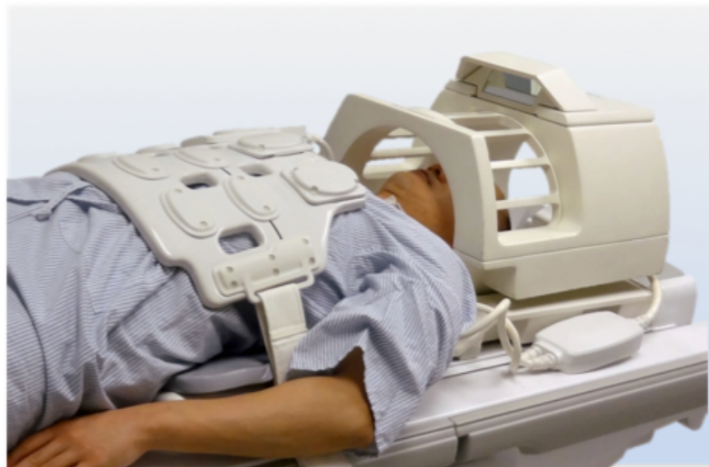
Figure 1.14: Traditional head and current flexible cardiac coils on patient.
