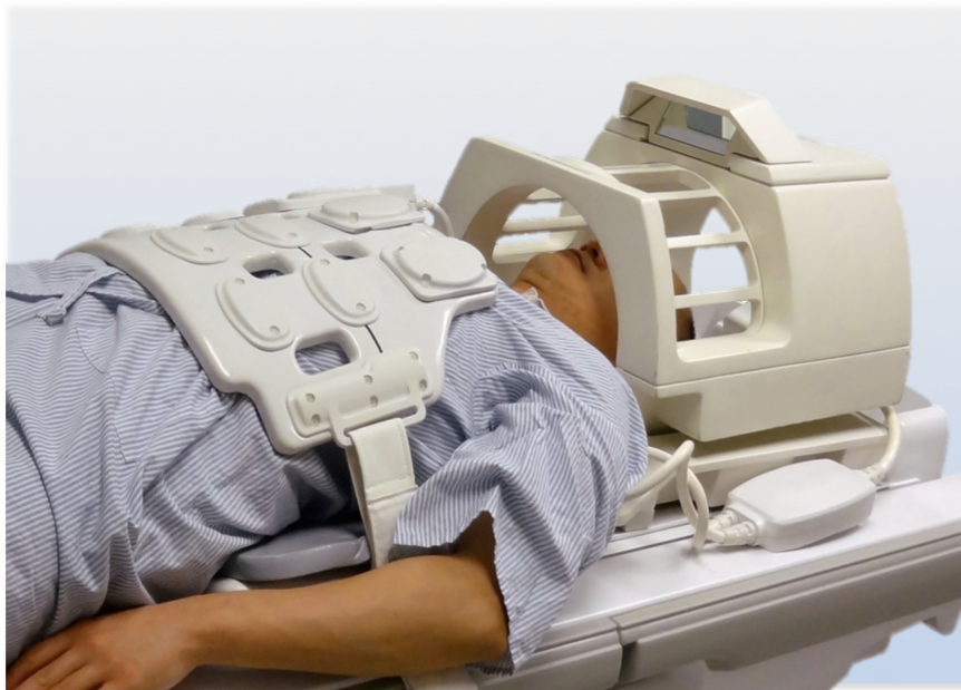
Figure 3.1: Two separate conventional MRI receive arrays on the chest and head of a patient.
