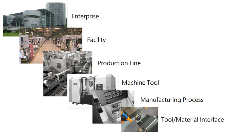
Figure 1.2: The spatial scope of manufacturing system (Derived from Dornfeld [23])
