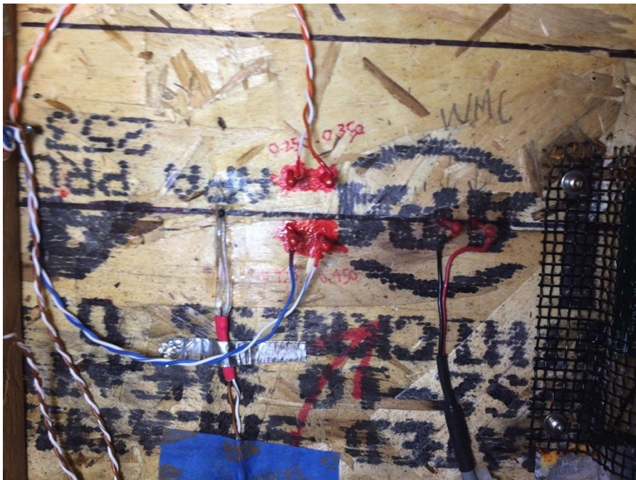
Figure 19 EW52 Fresno. WMC moisture pins, plus center-of-wood moisture pins, installed 2017-04-04.
