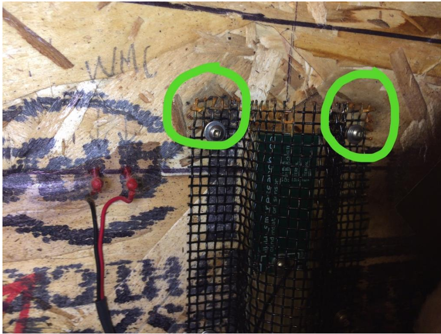
Figure 56 Fresno test home, rusted metal mesh at the North ridge location in the EW52 attic during interim inspection in April 2017.
