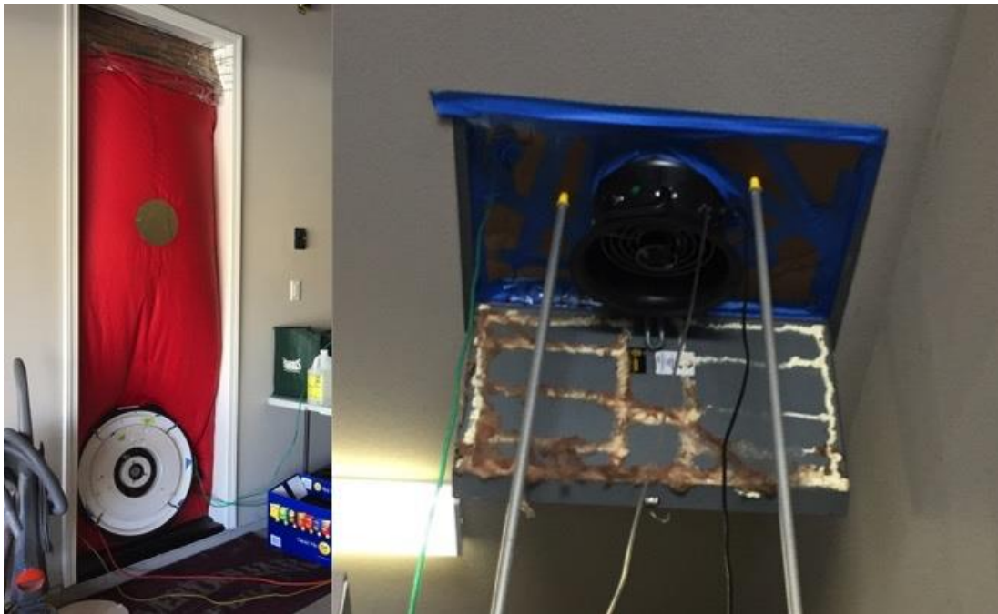
Figure 26 Two-fan test setup with blower door mounted in living space entrance and duct blaster fan mounted in attic access door.
