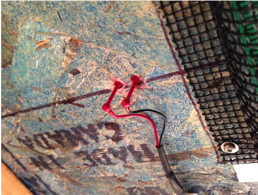
Figure 19 EW52 Fresno. WMC moisture pins, plus center-of-wood moisture pins, installed 2017-04-04.
