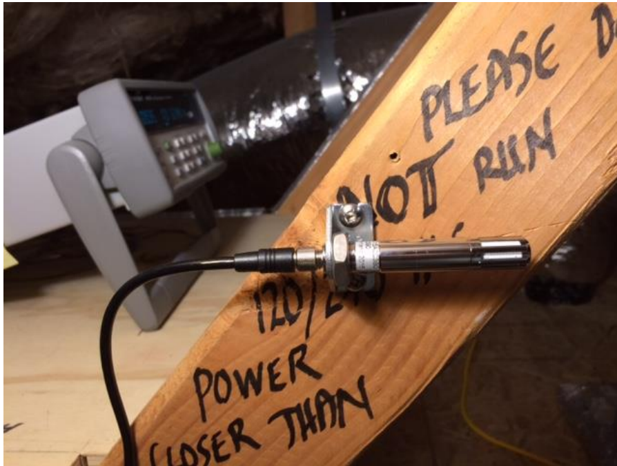
Figure 22 EW26N Clovis. Relative humidity and condensation sensors installed prior to placement of insulation.
