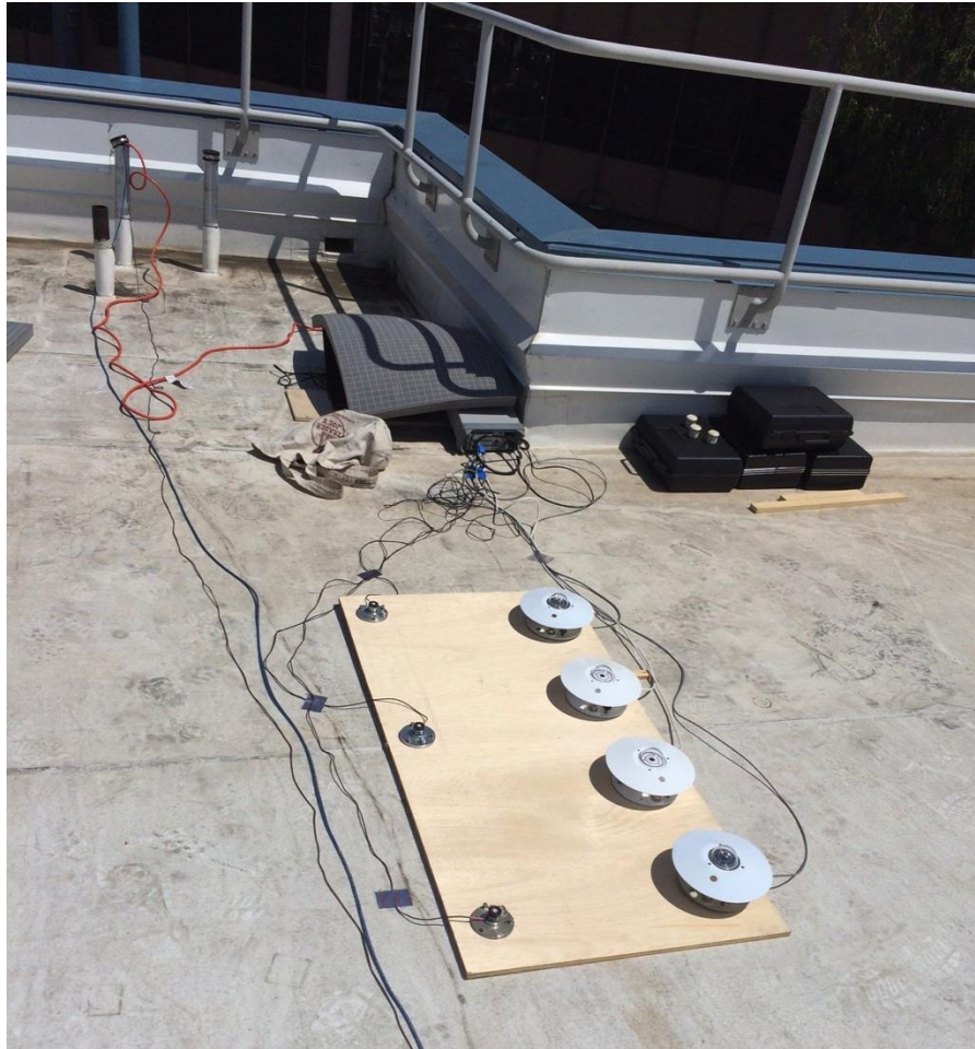
Figure 23 Cross-calibration of Eppley PSP and Licor pyranometers at LBNL prior to deployment.
