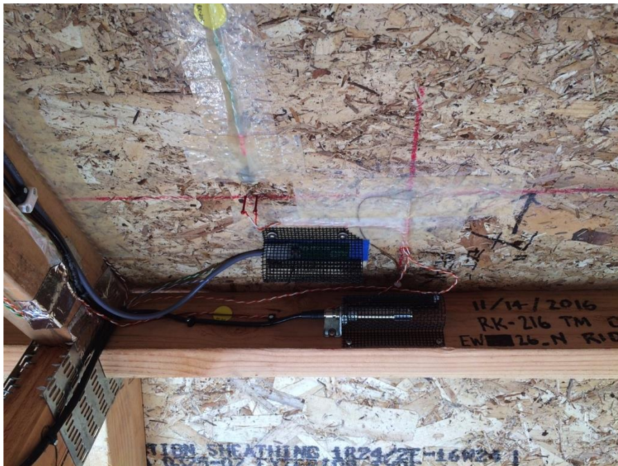
Figure 22 EW26N Clovis. Relative humidity and condensation sensors installed prior to placement of insulation.
