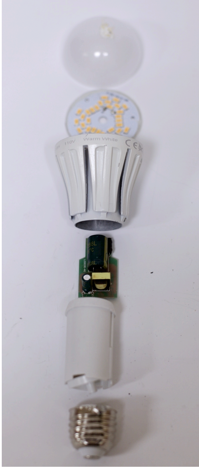
Figure 24: P03 product with removable fasteners and limited adhesives
