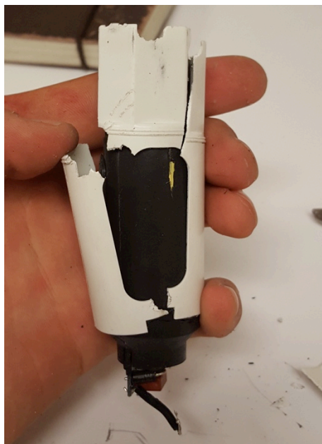
Figure 17: P15 Challenging Access to Driver
