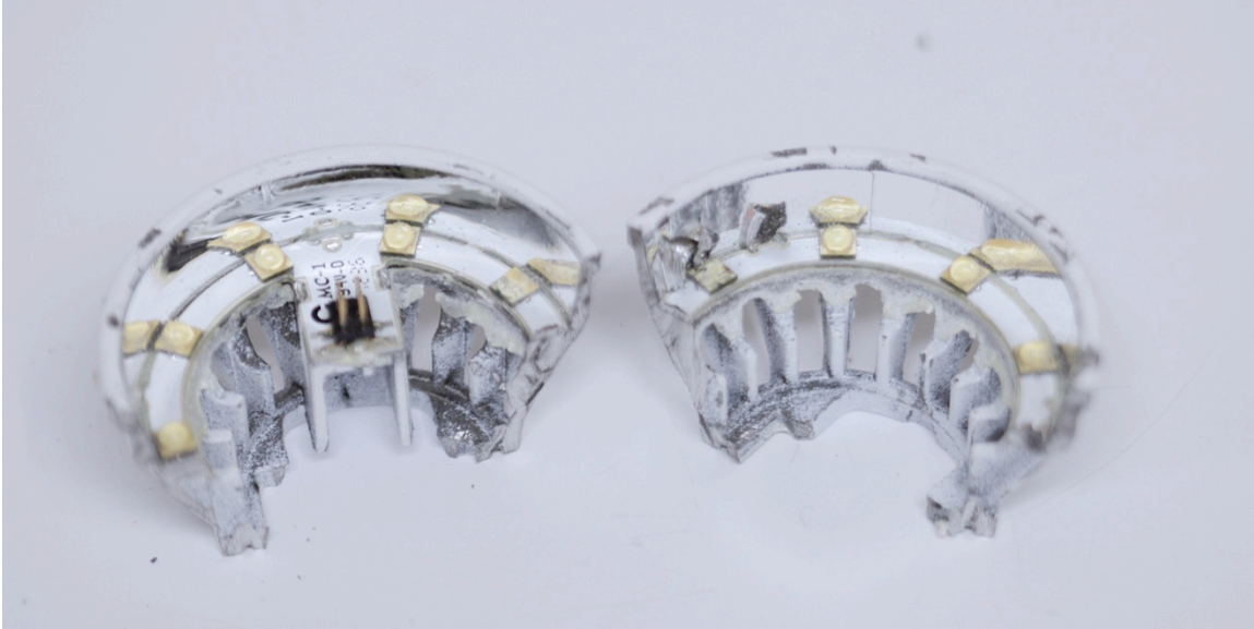
Figure 20: P02 product disassembly with heat exchanger in two parts. The sections required a Dremel tool for separation
