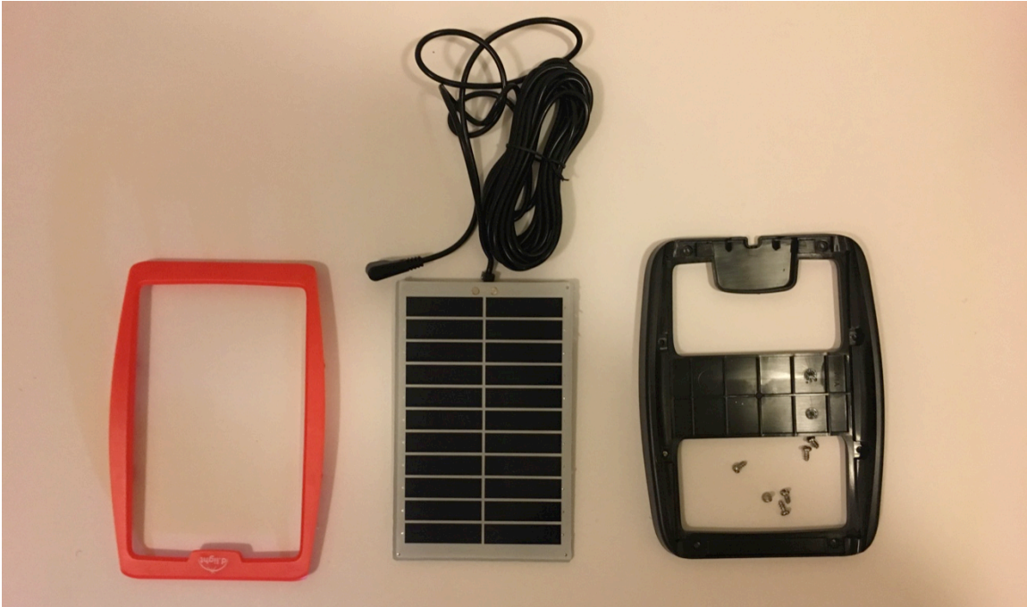
Figure 29: S01 Solar Charger as Example of Modular Design
