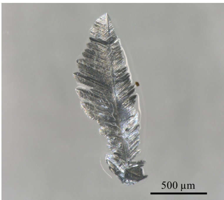
Figure 4.2, Optical micrograph of an electrodeposited Zn leaf acquired during oscillatory growth from 0.1 M ZnSO 4 (pH = 3.0) at a constant applied potential E = -2.0 V.
