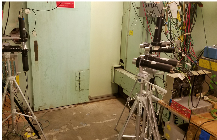
Figure 5.3: The detector array at the experimental area of the 88-Inch Cyclotron. On the left are the two target detectors mounted horizontally and a tertiary target not analyzed or discussed in this work. On the right are the six scattering detectors that observe the neutrons scatter out of the target detectors.
