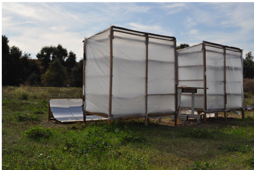
Fig. 4. Dryer 2 (left) is exposed to the concave solar concentrator. Dryer 1 (right) is the control.
