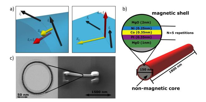
**Figure 1.** a) Effective DMI for neighboring spins on curved (left) and planar (right) surfaces. b) Schematic layout of the magnetic multi-layered nanotube. c) Cross-sectional bright-field STEM (left) and SEM (right) image of the deposited nanotube.
