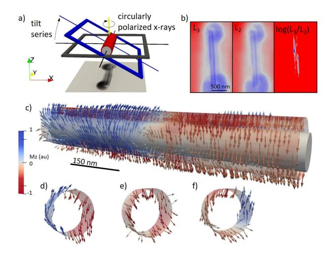
Figure 2. Magnetic soft x-ray tomography a) Schematics of the experimental setup, b) Raw experimental data recorded at the  $L_3$ ,  $L_2$  edges, and corresponding difference signal, c) Reconstructed 3D spin texture, d) - f) Slices from the reconstructed data taken at both ends d), f) and at the transition region e).
