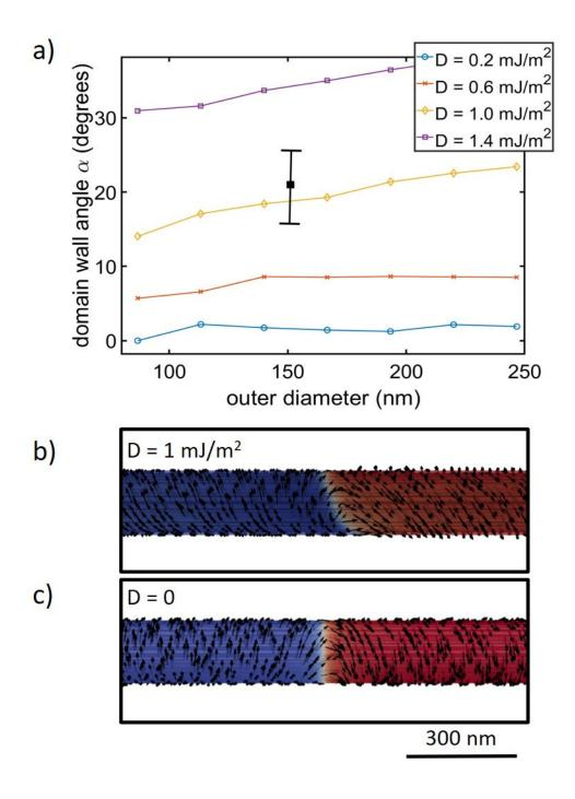
**Figure 4. Quantitative analysis of the DW angle.** a) Domain wall angle to nanowire axis as function of outer diameter for different DMI values. b) Simulated domain wall with DMI. c) Simulated domain wall without DMI.
