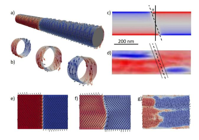
Figure 3. Simulation and comparison with experiment: a) Rendering of simulated nanotube magnetization. b) Slices showing the opposite chiralities on both ends and the transition region. c) Z-axis projection of simulated magnetization, d) Z-axis projection of experimental data. Dashed lines in c) and d) indicate the inclination of the domain wall (dotted line is experimental error). e), f) and g) Digitally unwrapped simulation of the nanotube e) without DMI, f) with DMI and g) experimental data.
