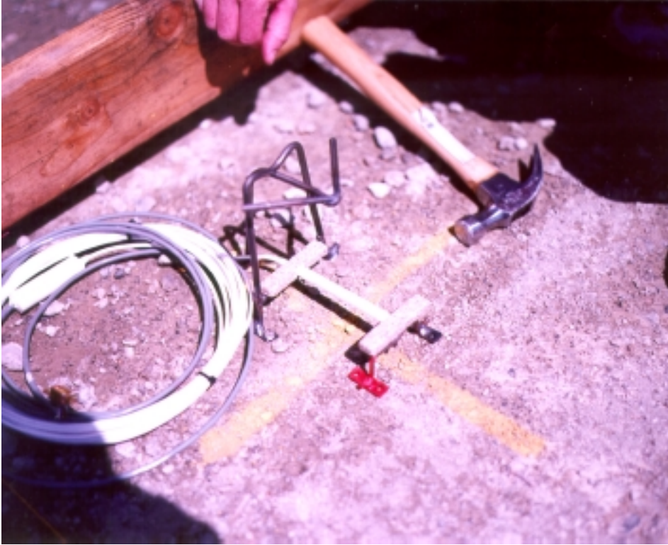
Figure 6.5. Steel Frames for Collocation of Dynatest PAST-2PCC (shown) and Tokyo-Sokki PMR-60-6L (not shown).
