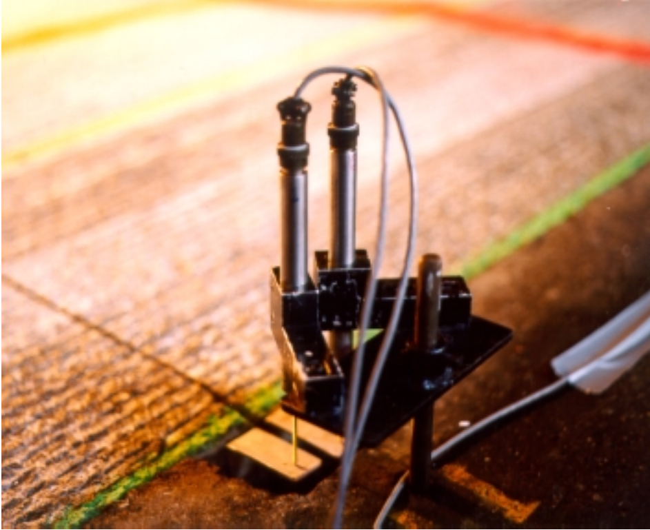
Figure 6.24. Joint Displacement Measuring Device (JDMD) on South Tangent. ( Edge Displacement Measuring Device is essentially identical except that it is placed in the middle of the slab instead of at the joint. )
