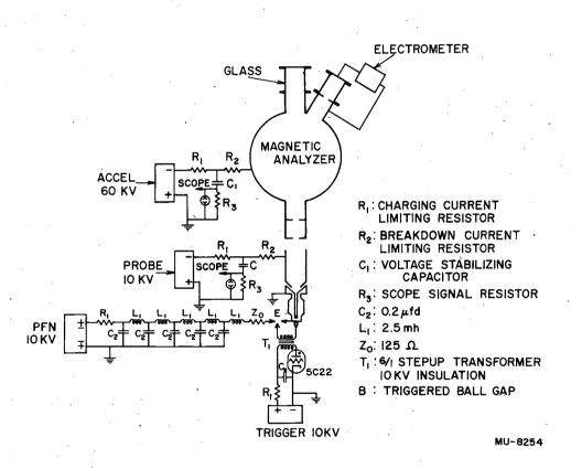
Fig. 3 300- $\mu$ sec source test setup.
