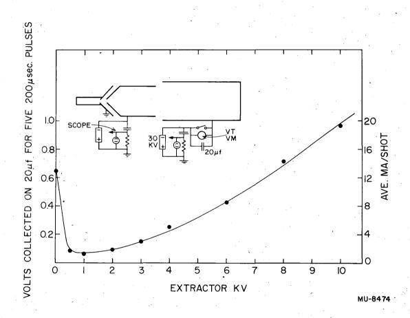
Fig. 4 Collector beam vs extractor voltage.
