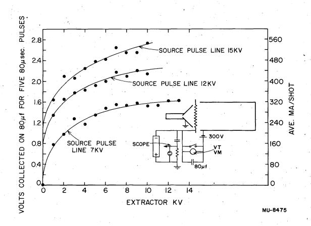
Fig. 5 Collector beam vs extractor voltage.
