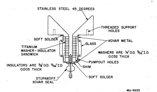
Fig. 2 Cross section of "inside" washer source.
