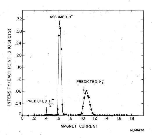
Fig. 6 Distribution of ions from H source with 35 kv accel.
