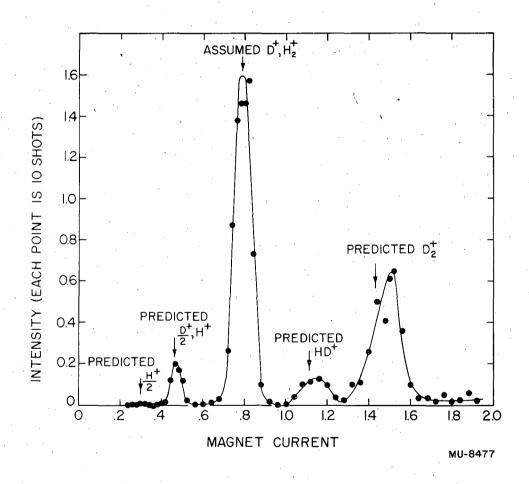
Fig. 7 Distribution of ions from D source with 36 kv accel.
