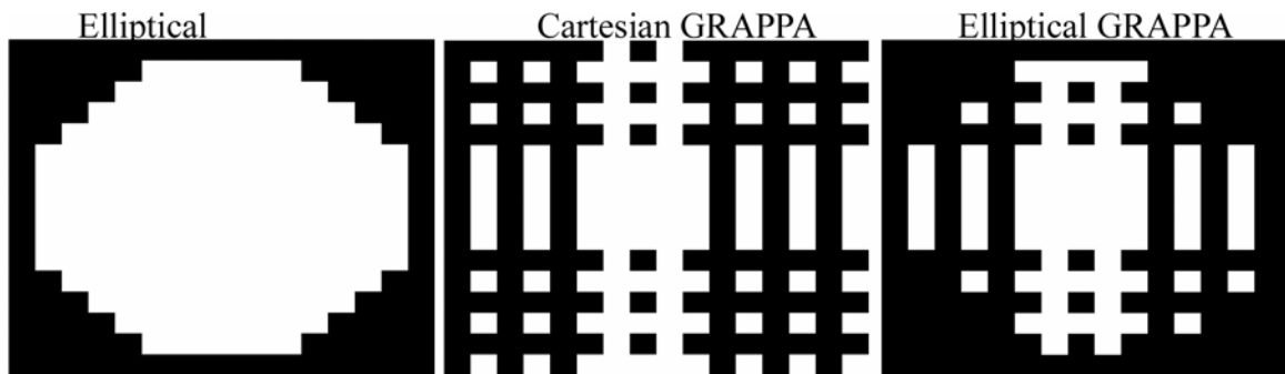
Fig 7.2 shows the sampling schemes in k_x - k_y plane for 16x16 Elliptical, Cartesian GRAPPA and Elliptical GRAPPA methods
