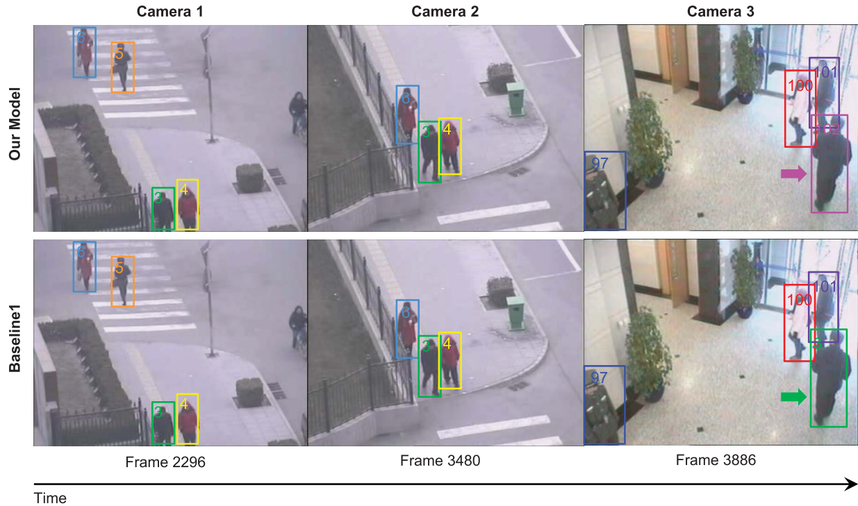
Fig. 8. Visual comparison of our model (the first row) and Baseline1 (the second row) on Dataset1. It is observed that Baseline1 mistakenly identifies a new target in Camera 3 (the one pointed by arrow) as target 3, while our model avoid this error by maintaining the group consistency between targets 3 and 4. Bounding box with the same color indicates the same target. Best viewed in color.
